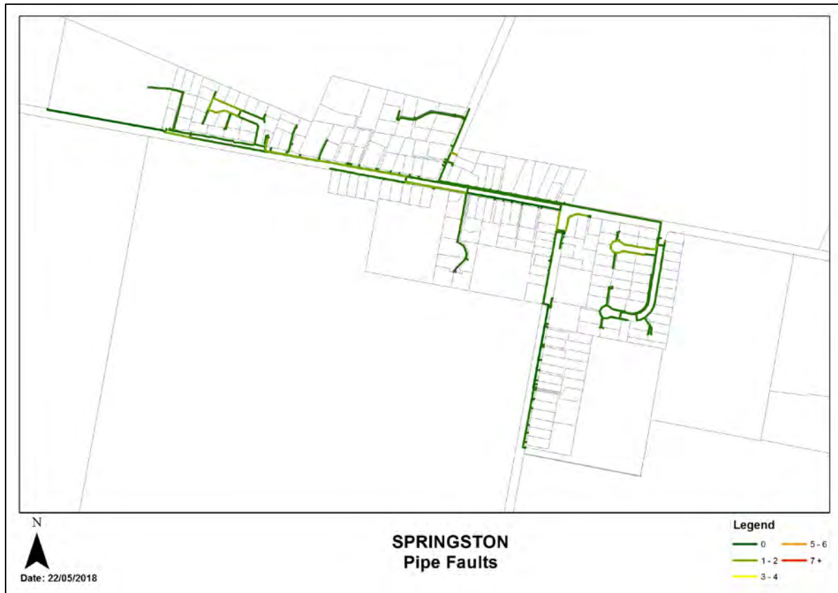
Figure 23-9 Pipe Faults, Springston
