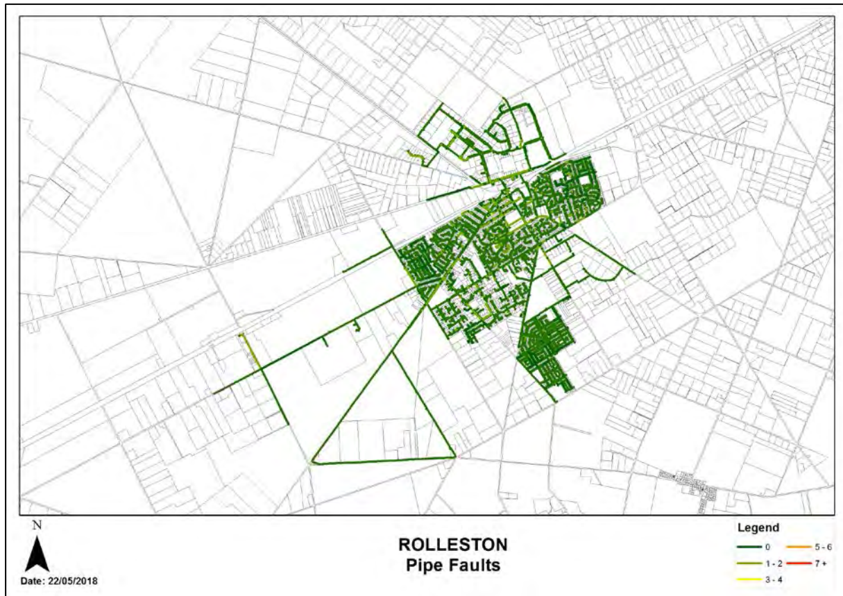
Figure 19-14 Pipe Faults, Rolleston
